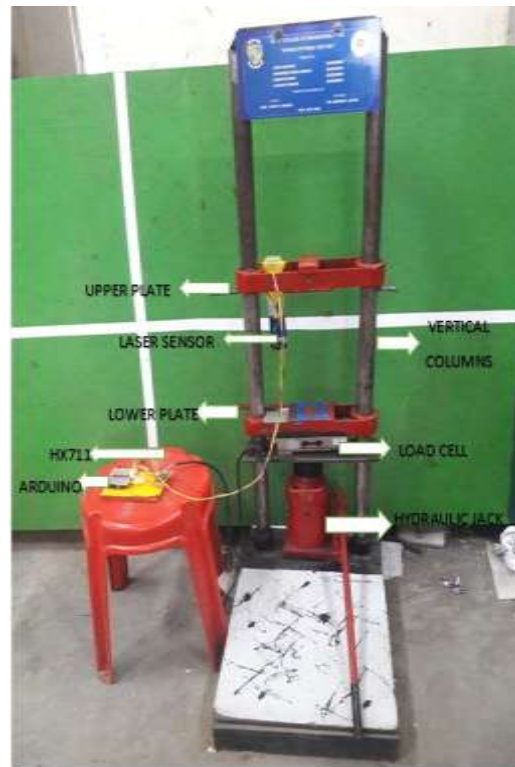
Fig.1 Spring Stiffness Test-rig
